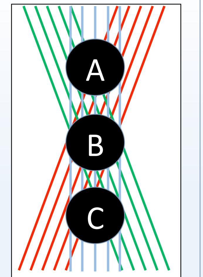
Figure 2. The orientation of detectors, A, B, and C. The lines indicate the detection window. Only when a particle passes through at least two of the detectors does it trigger a muon
