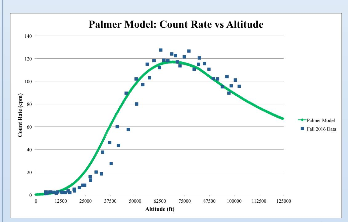
Figure 1. Muon count versus altitude. The blue data points were collected during a balloon flight in the fall of 2016. The green line is a mathematical model developed by Michael Palmer.
