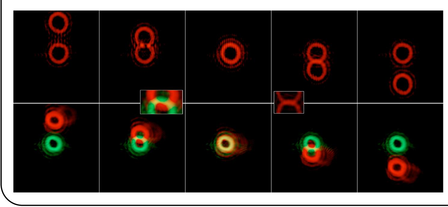
By using colored filters in front of the SLM, monochromatic vortices can be easily generated. The phase tilt encoded into each forked pattern can be smoothly varied, allowing for independent, real-time control of the vortices. Here, two red vortices exhibit interference as they pass through each other, while a red and green vortex beam pass through each other without interference.
