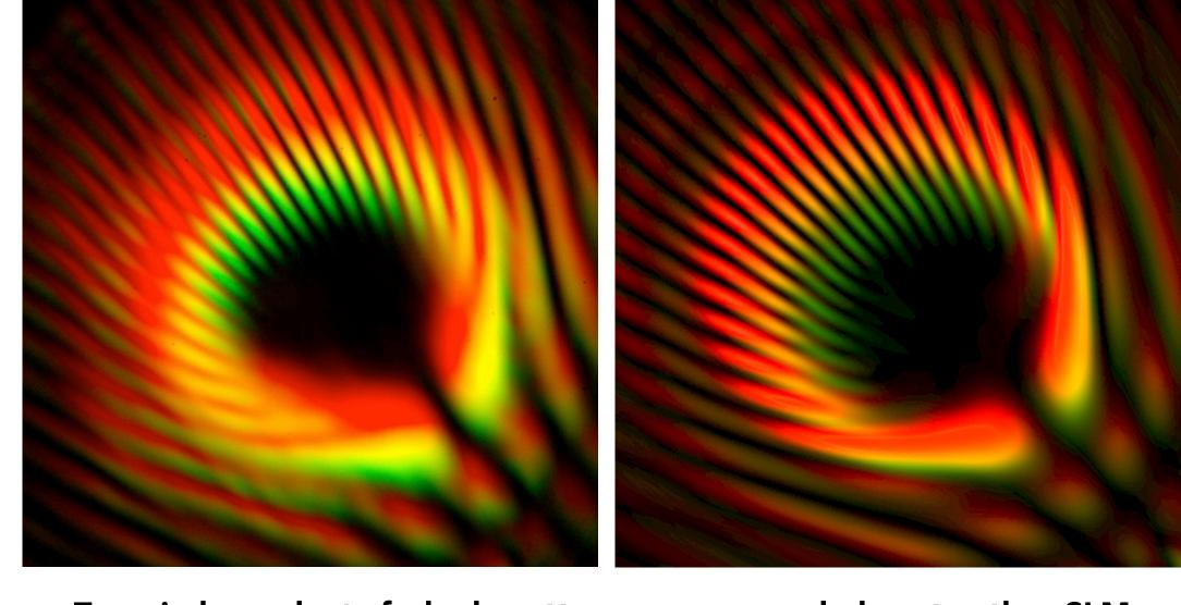
Two independent forked patterns are encoded onto the SLM, simultaneously generating two broadband vortices that are made to interfere on the CCD. Here, the brilliant interference pattern generated with vortices of opposite topological charge (+10, -10) are captured in full color with a Nikon D70s DSLR camera (left panel). Numerical calculations (right panel) show excellent agreement.
