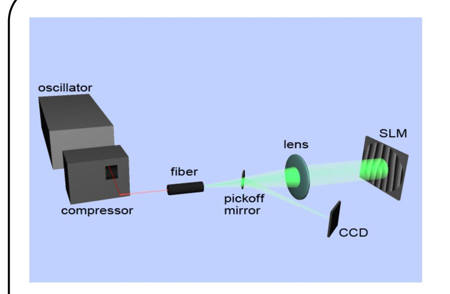
Pulses generated with the Ti:S oscillator are optimized with a pulse compressor and injected into the "holey" fiber, generating a diverging beam of supercontinuum light. An f=70cm lens collimates the light before it strikes the SLM. The reflected light is refocused by the lens onto a CCD via a pickoff mirror.
