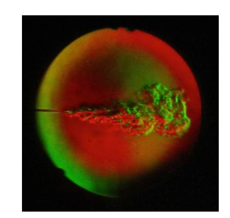
Air flow from a compressed air can is imaged with the two-path, double knife edge system.
