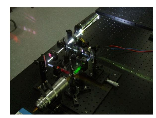
The white light from the LED passes through both arms of the apparatus, complete with red and green color filters.
