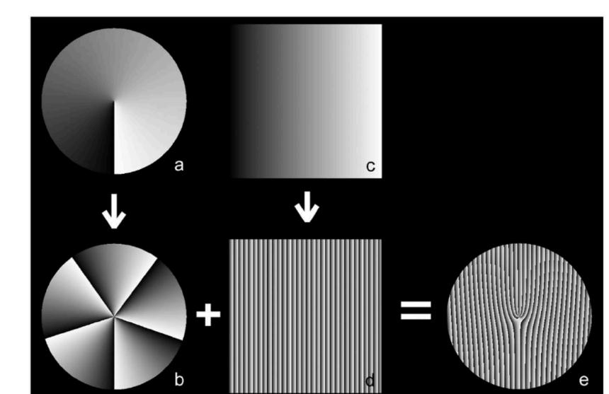
It is important to note that by encoding the phase pattern and diffraction grating together on the SLM, that only the properly shifted portion of the beam will be diffracted to the first order, regardless of the calibration of the device. This is a crucial point when shaping ultrabroadband light, and allows for excellent vortex generation for all colors within the super-continuum.
