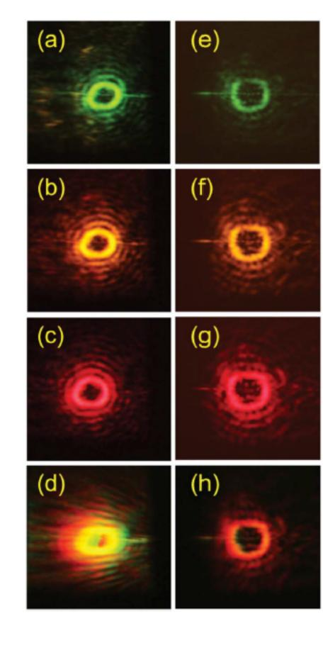
True-color images of doubly dispersed (left column) and dispersion-corrected (right column) vortices are shown for 550nm (a,e), 580nm (b,f), 619nm (c,g) and the full spectrum (d,h). The full-spectrum case clearly demonstrates the severe spatial chirp in the doubly dispersed case and the excellent overlap in the dispersion-corrected case.
