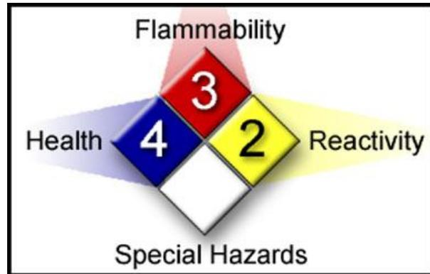
The NFPA hazards are rated with 0 as the least, and 4 as a significant hazard. Additional information is provided below:
