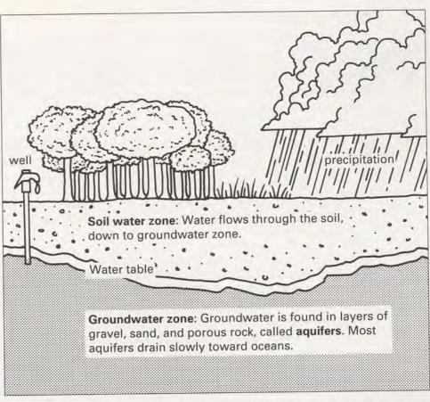
Figure 2 Model of groundwater system, showing how groundwater is obtained (wells) and recharged (precipitation and snowmelt).
