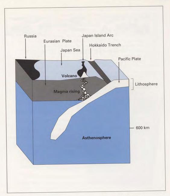
Figure 2 Diagram of a subduction zone. East of the island of Hokkaido, Japan, the Pacific Plate slides below the Eurasian Plate at an angle of 45° and extends toward the Asian mainland. This subduction passes underneath Hokkaido, causing earthquakes to occur along the zone to a depth of 600 km. Shallow earthquakes, which usually cause the greatest damage, occur in the overriding Eurasian Plate.
