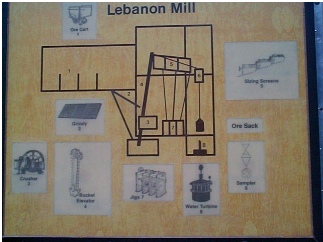
Process of milling ore
