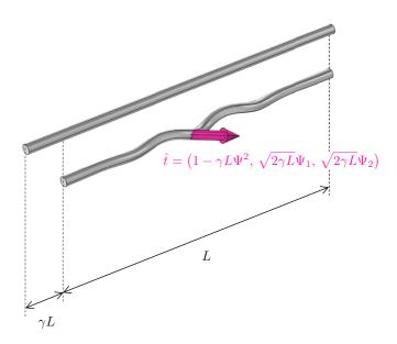
FIG. 1. Arbitrary small 3D deformation produced by subjecting a straight inextensible rod (oriented along  $\hat{x}$ ) to a relative compression  $\gamma$  (shown greatly exaggerated). The vector function  $\vec{\Psi} = \Psi_1 \hat{y} + \Psi_2 \hat{z}$  appearing in the expression for the rod's unit tangent vector  $\hat{t}$  satisfies a squared Schrödinger equation [Eqs. (7)] as well as a normalization-like constraint.
