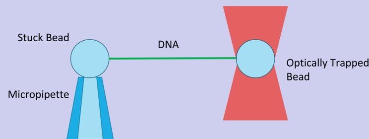
DNA can be stretched by fixating one protein coated bead with a micropipette, and pulling on another bead with the optical tweezers. DNA will be attached to both beads using two proteins: biotin and streptavidin.
