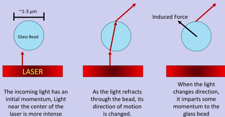
A gradient laser intensity generates unsymmetrical forces on the object, making the total force directed towards the center of the laser beam. This inward force can be modeled as a simple harmonic oscillator, providing a way to measure external forces using the position of the bead relative to the laser center. This approximation is governed by the equation:
