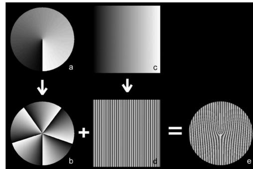
It is important to note that by encoding the phase pattern and diffraction grating together on the SLM, that only the properly shifted portion of the beam will be diffracted to the first order, regardless of the calibration of the device. This is a crucial point when shaping ultra-broadband light, and allows for excellent vortex generation for all colors within the super-continuum.
