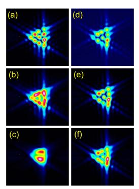
Fig. 8. (Color online) False-color diffraction patterns in the near infrared from a 0.73 mm triangular aperture of charge 3 vortices. The left column shows the doubly dispersive case for (a) cw, (b) femtosecond, and (c) supercontinuum modes. The right column shows the dispersion-corrected case for (d) cw, (e) femtosecond, and (f) supercontinuum modes.
