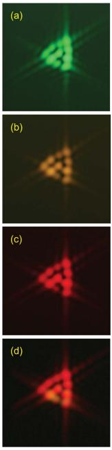
Fig. 9. (Color online) True-color diffraction patterns in the visible for a charge 3 supercontinuum vortex from a 0.73 mm triangular aperture: (a) 523 nm, (b) 580 nm, (c) 620 nm, and (d) full spectrum.
