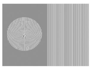
Fig. 5. Screenshot of the grayscale pattern displayed on the SLM. The left half of the SLM displays an apodized forked grating for generating a vortex beam. The right half displays only a blazed grating.
