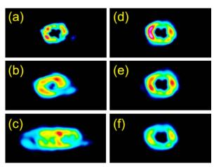
Fig. 6. (Color online) Charge 3 vortex is generated in the doubly dispersive case for (a) continuous wave (CW), (b) femtosecond (fs), and (c) supercontinuum (NIR SC). The dispersion-corrected case is shown for (d) CW, (e) fs, and (f) NIR SC.
