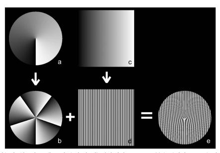
Fig. 1. Spiral phase combined with a phase tilt results in the familiar forked phase pattern. (a) A spiral phase ranging from  $0-10\pi$  is (b) displayed modulo  $2\pi$ , resulting in a phase plate with five  $0-2\pi$  segments. Likewise, (c) a phase tilt is (d) displayed modulo  $2\pi$ , resulting in a blazed grating. The addition of these two patterns results in (e) a forked phase pattern.
