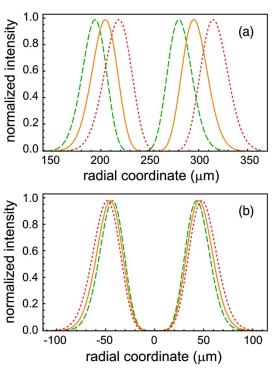
Fig. 3. (Color online) Calculated cross sections of optical vortices (charge m=3) emerging from the (a) doubly chirped and (b) zero-chirp optical system. The three vortices shown in both cases correspond to the wavelengths 550 nm (dashed green line), 580 nm (solid orange line), and 619 nm (dotted red line). For the calculations, we used f=70 cm,  $w_0=173~\mu\mathrm{m}$ , and grating period  $d=325~\mu\mathrm{m}$ . These parameters were chosen to approximate the conditions of our experiment.
