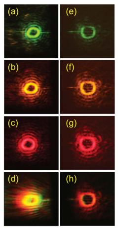
Fig. 7. (Color online) Color vortices are recorded with a color DSLR CCD array. The left column shows the doubly dispersive results at wavelengths (a) 550 nm, (b) 580 nm, (c) 619 nm, and (d) full spectrum. The right column shows the dispersion-corrected results for (e) 550 nm, (f) 580 nm, (g) 619 nm, and (h) full spectrum.
